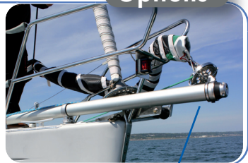
Articulating toggle for Gennaker / Code zero furler attachment,
