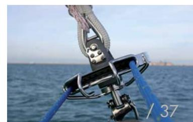
\* The S.W.L. is the maximum safe working load over which distortions of the furler can appear. This load is approx. 50% of the breaking load (depending on models)
